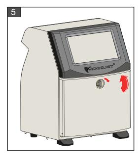
5. Close the ink compartment door. Rotate the horizontal knob in clockwise direction to vertical position to lock the ink compartment door.
