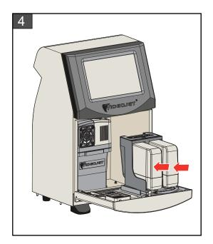
Insert the ink cartridge/make-up fluid into the cartridge holder by aligning the cartridge key with the correct holder slot.
