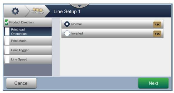
Figure 6-30: Line Setup - Printhead Orientation
