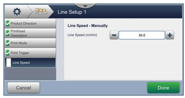
Figure 6-36: Line Speed - Manual Setup
