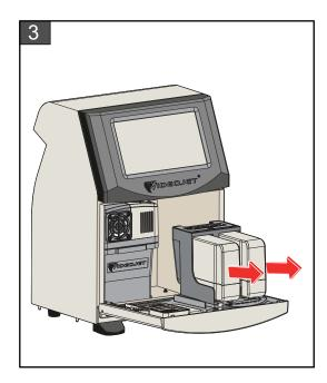
**3.** Pull the old (ink and/or make-up fluid as needed) cartridge to remove it from the cartridge holder.
