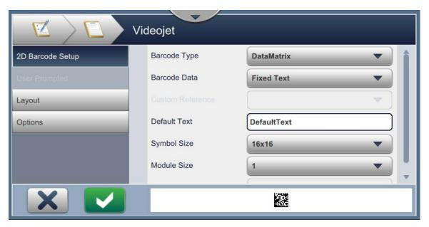
Figure 6-10: 2D Barcode Setup Screen
