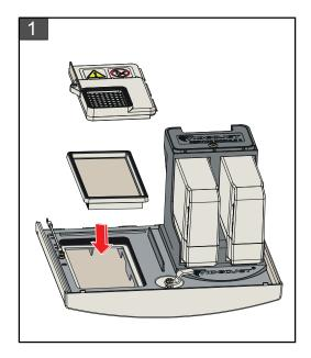
**1.** Insert the new Air Filter element and Air Filter cover.
