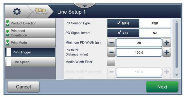
Figure 6-34: Line Setup - Print Trigger
