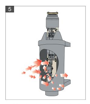
5. Allow the printhead to dry and make sure that the slot in the charge electrode is free of cleaning solution. Remove the printhead from the wash station.
