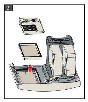
**3.** Remove the Air Filter cover and Air Filter element from the door.
