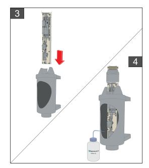
**3.** Put the printhead into the wash station with a properly earthed bowl underneath.
