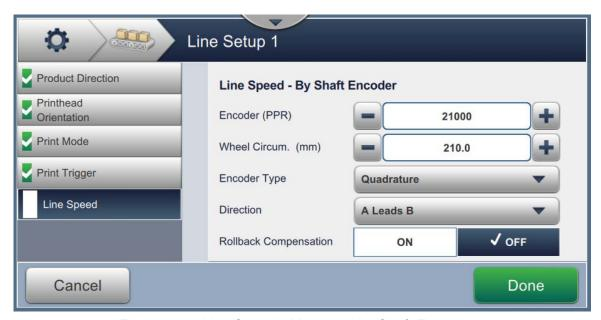
Figure 6-37: Line Speed - Measured by Shaft Encoder
