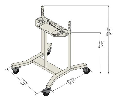
Figure A-2: Mobile Printer Stand
